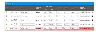
For the (2) Sensor disconnected scenario, you can also define an alert, -999.9 degrees Celsius means sensor not found and the device can alert you of this situation.
